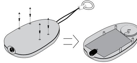
Should you need to replace the battery in the remote control, simply identify and unscrew the four screws on the underside of the remote control. Once the screws have been removed, the remote control will come apart and reveal the 'button cell battery'. Remove the battery and replace with a new battery that matches the specifications of the one removed. Observe correct polarity when inserting the battery and screw the remote control back together.
