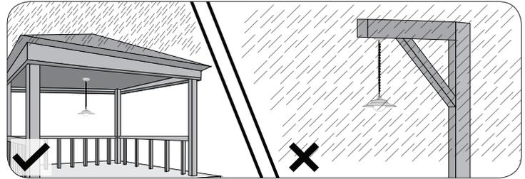
The solar hanging light is not weatherproofed. Only mount the hanging light in a dry environment not exposed to the elements.
