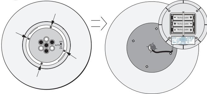
Should you need to replace the light's batteries, simply unscrew the dome. You will then have access to 4 screws around the edge of the light. Once you have unscrewed and lifted the LED light fitting, you will see the batteries.
