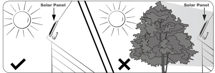
Ensure your solar panel is placed so that its exposure to the sun is optimized. Be aware of objects such as trees or property overhangs that may impede the panel's ability to generate a charge.
