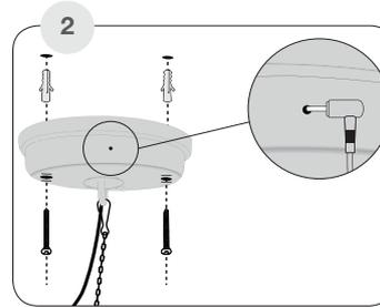
Install the ceiling mount with integrated chain to your chosen surface using the two remaining mounting screws and wall plugs (if required). Ensure the sensor on the ceiling mount is unobstructed as it could limit the remote control's ability to operate.
