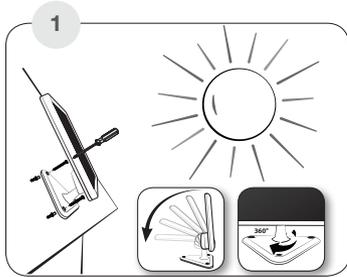
The angle of the solar panel can be adjusted utilizing the pivot point where the solar panel attaches to the bracket. This allows you to maximize sun exposure.
