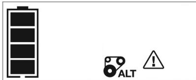
The Battery Status Icon, Alternator Icon and "ALT" will light solid. The Fault Icon will flash.
