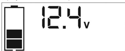
The bars on the Battery Status Icon represent the charge level of the unit's internal battery. The bars on the Battery Status Icon will change from empty to solid (bottom to top) repeatedly to indicate the unit is charging. The backlight will turn on for 10 seconds (only).
