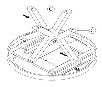
Assembly using 2" bolts (2), lock washers (3), and flat washers (4). Tighten all bolts fully.
