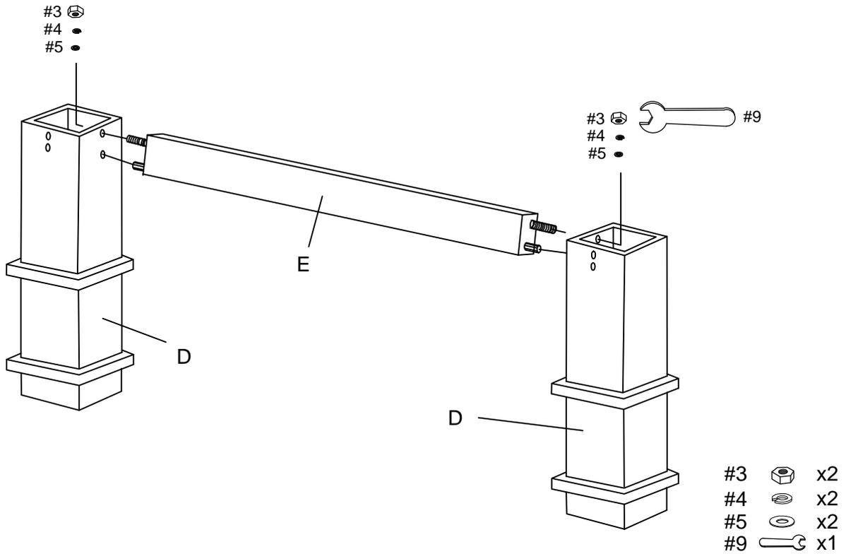
Step 2 . Attach table supports (part F) to pedestals (part D) using large flat washers (part #5), large spring washers (part #4), hex nuts (part #3) and wrench (part #9).
