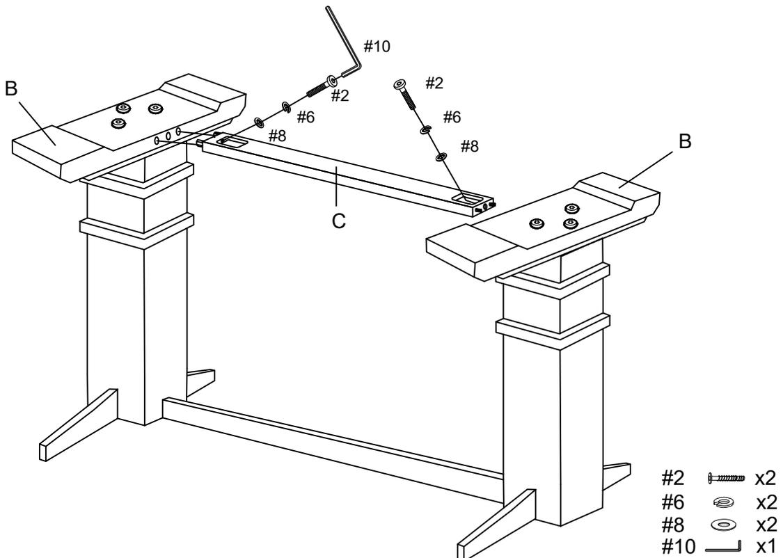
Step 5 . Lay table top (part A) upside down on a soft surface, such as carpet. Attach assembled unit (parts E & F) to table top (part A) using small flat washers (part #8), spring washers (part #6), short bolts (part #2) and allen wrench (part #10).
