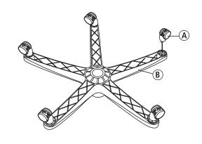
**Step 2**Turn the Star Base (B) over and insert the Gas Lift with Telescoping Cover (C) through the center hole on top of Star Base (B).
