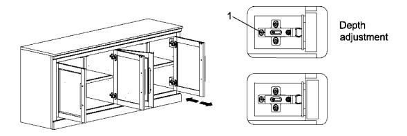
1) Loosen or tighten the indicated screw to adjust the gaps forward and backward between doors and console.
