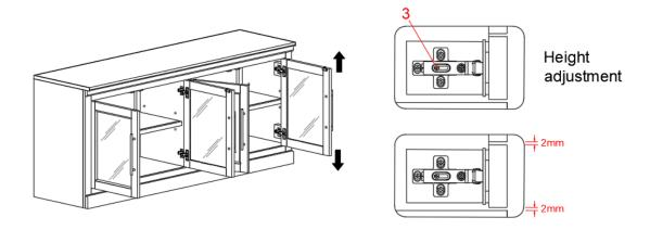
3) Loosen or tighten the indicated screw to adjust the door vertically to the desired position.
