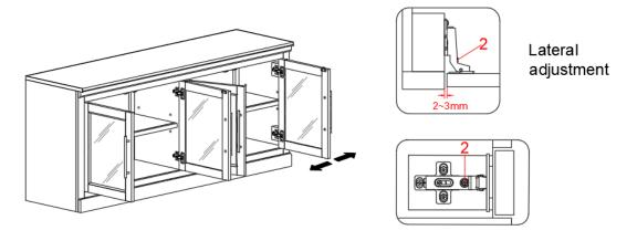
2) Rotate the screw clockwise or counterclockwise to adjust the door horizontally as shown.
