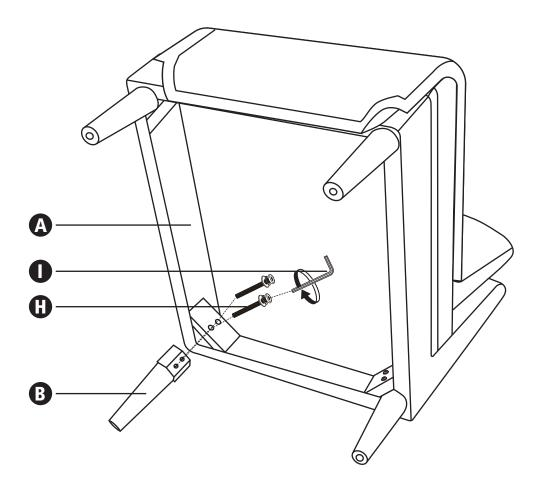
Attach legs (B) to the four corners of the chair (A) using 5/16"x 2%" L bolts with washers for chair (H) by allen key (I) as shown.
