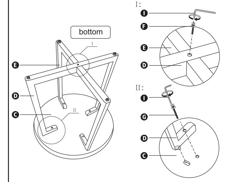
Attach table leg (D) to the table top (C) using 1/4" x 2" L bolts with washer (G) and 1/4" x 11%" L bolts with washers (F) to table leg (E), tighten with allen key (I).
