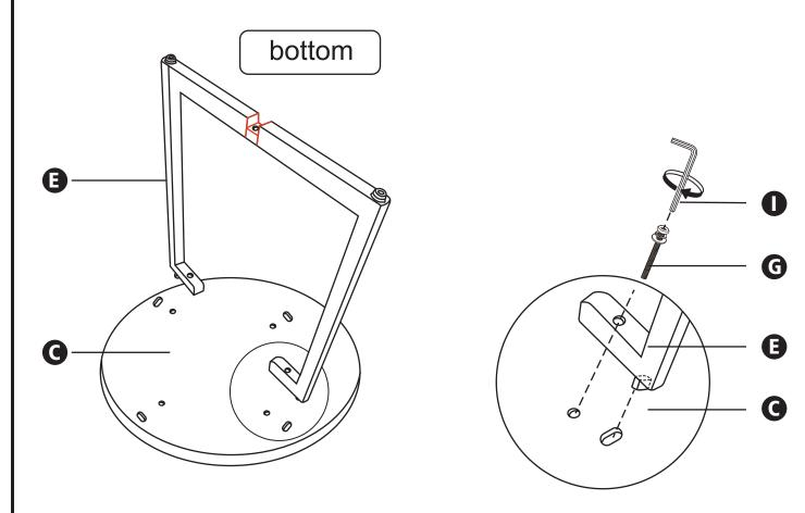
Attach table leg (E) to the bottom of the table top (C) using 1/4"  $\times 2$ " L bolts with washers for table (G) by allen key (I) as shown.
