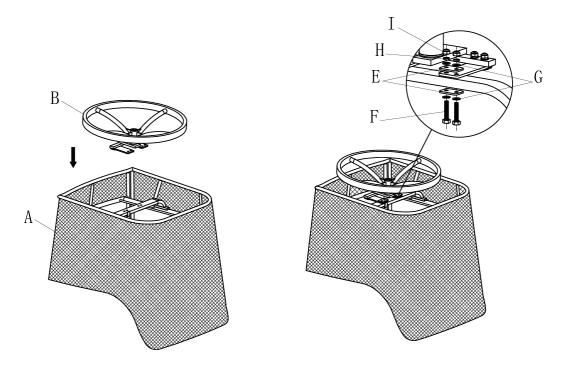
Carefully place chair frame(A) upside down a soft, flat and non-abrasive surface. Attach the chair base (B) to chair frame (A) using M8 bolts(F), Washer(G), Spring washer (H) and M8 Damping nuts (I).
