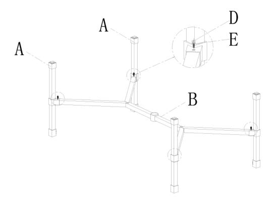
Assemble the table legs (A) to table support bar (B) with M6 bolts (D) and M6 washer (E) by using M6 Allen wrench (I).
