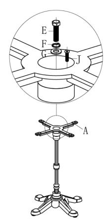
Assemble the X Support frame (A) and leg (B) M12 bolts (E), M12 Spring Washer (F) and M12 Washer (G) by using M12 Hex wrench (L).
