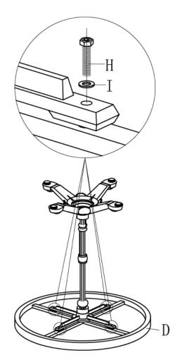
Carefully place the table top (D) upside down on a non-abrasive surface. Assemble the table top (D) to the X support frame (A) with M6x30mm bolts (H) and M Washer (I) by using M6 Allen wrench (J).
