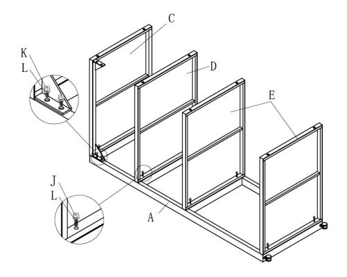
Carefully place the Left leg frame (A) upside down on a non-abrasive surface. Assemble the Shelf 1 (C), Shelf 2 (D) and Shelf 3 (E) to Left leg frame (A) with M6 bolts (K), M6 bolts (J) and M6 Washer (L) by using M6 Allen Wrench (M).
