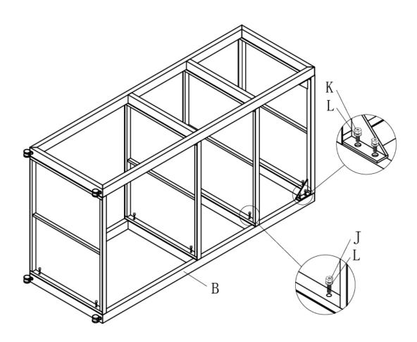
Assemble the Shelf 1 (C), Shelf 2 (D) and Shelf 3 (E) to Right leg frame (B) with M6 bolts (K), M6 bolts (J) and M6 Washer (L) by using M6 Allen Wrench (M). Tighten all bolts with M6 Allen Wrench (M).
