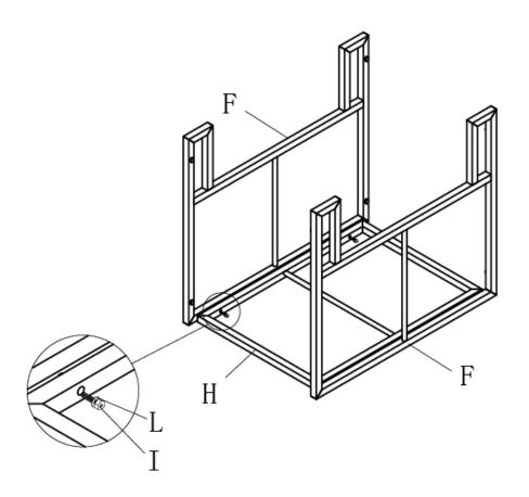
Assemble the Woven panel 1 (F) to Woven panel 3 (H) with M6 bolts (I) and M6 Washer (L) by using M6 Allen Wrench (M).
