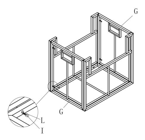
Assemble the Woven panel 2 (G) to Woven panel 3 (H) with M6 bolts (I) and M6 Washer (L) by using M6 Allen Wrench (M). Tighten all bolts with M6 Allen Wrench (M).
