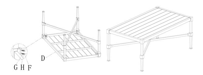
Carefully place the table top (D) upside down on a non-abrasive surface.
