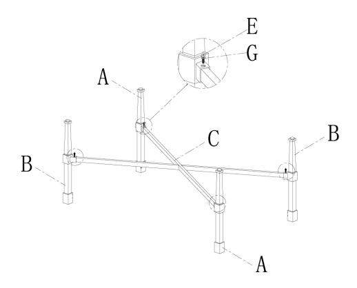
Assemble the table legs 1 (A) and table legs 2 (B) to table support bar (C) with bolts (E) and M6 washer (F) by using Allen wrench (I). Do not tighten the bolts until assembling is completed.
