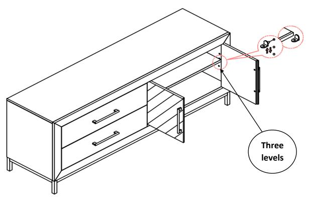
• If you want to remove, please lift the shelf a little bit (1) and pull out the shelf pin – work with all the shelf pins until you can align. Then decide which level (2) you want by putting all the shelf pins into the hole. Adjust shelf to balance.
