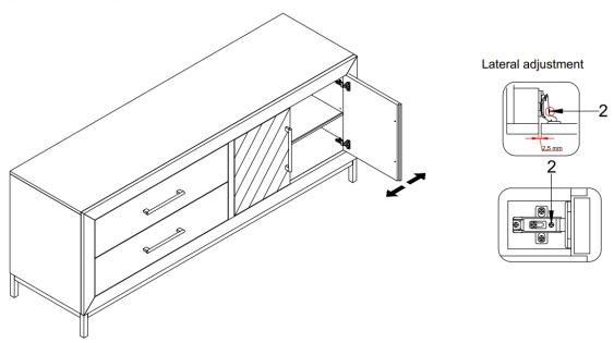
2) Rotate the screw clockwise or counterclockwise to adjust the door horizontally as shown.
