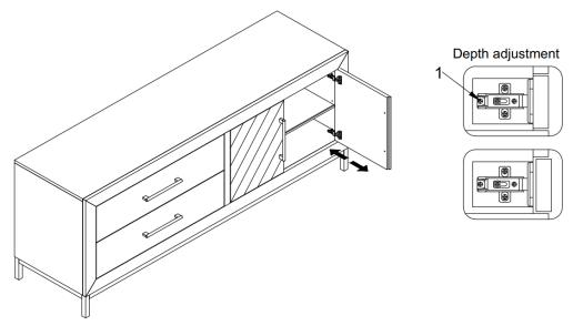
1) Loosen or tighten the indicated screw to adjust the gaps forward and backward between doors and console.
