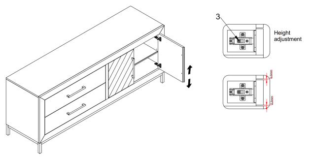
3) Loosen or tighten the indicated screw to adjust the door vertically to the desired position.
