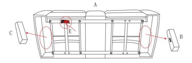
Step 3: Plug the 3 Chair Back (D) into the Chair Base (A) correctly and buckle the 1 Right Back Post (B) and 1 Left Back Post (C) on the the Chair Base (A) one by one.
