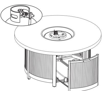
Please do not remove the chain from the fire pit base frame end or from the valve end when the valve is disconnected from cylinders.
