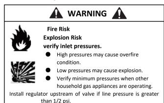
Pressure requirements for appliance are shown in table below. Minimum pressures must be met when other household gas appliances are operating.
