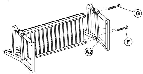
Attach the left side frame (A2) into the assembly from step 3. Secure with 1 3/4" bolts (F) and 2" bolt (G), using screwdriver.
