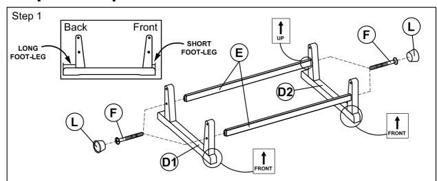
Attach base cross bars (E) into right and left base side frame (D1&D2) and secure using 1 3/4" bolts (F).
