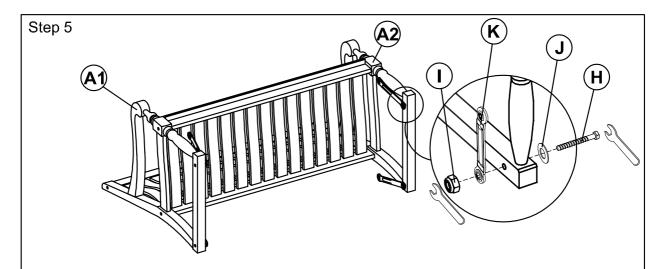
Assemble gliding stretches (K) into leg frames (A1&A2) and secure using 2 3/4" bolts (H), washer (J) and nuts (I) as diagram shown.
