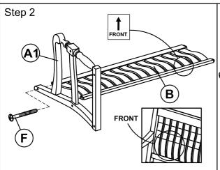
Attach the right side frame (A1) into backrest (B). Secure with 1 3/4" bolt (F).
