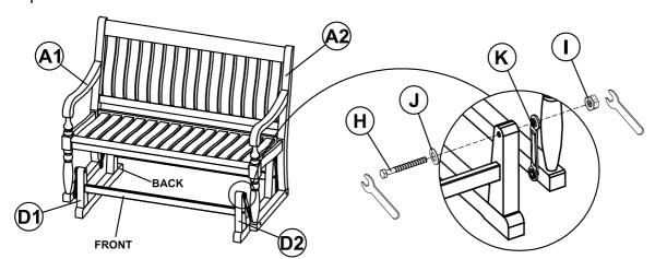
Attach the previously assembled base side frames (D1&D2) to the leg frames (A1&A2). Connect using gliding stretches (K) to the leg frames (A1&A2) and secure using 2 3/4" bolts (H), washers (J), nut (I) as diagram shown. Tighten the nuts and bolts using wrench.
