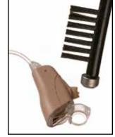
**To remove the battery,** open the door and push the battery up and away from the lipped side of the door or use the magnetic end of the utility brush to easily lift out the battery.
