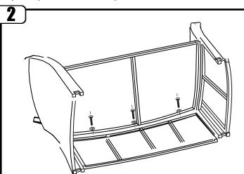
Attach seat panel to loveseat back by completely tightening 3 Bolts (A) and 3 Washers (D) as shown, with Hex Wrench (G) provided.
