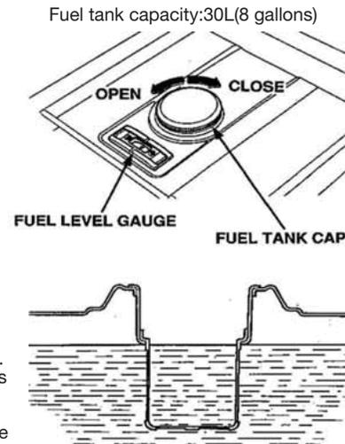
Use gasoline with a pump octane rating of 90 or higher. We recommend unleaded gasoline because it produces fewer engine and spark plug deposits and extends exhaust system life. Never use stale or contaminated gasoline or oil/gasoline mixture. Avoid getting dirt or water in the fuel tank.
