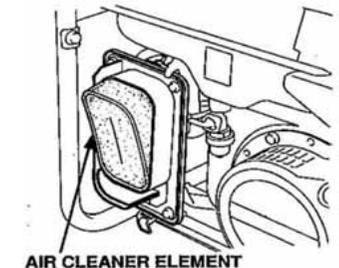
4. Reinstall the air cleaner element and the cover.
