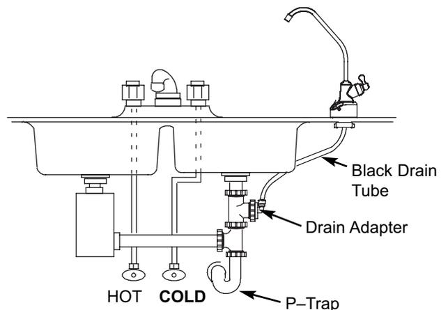
**IMPORTANT: Locate drain adapter so that when the black drain tube from the Reverse Osmosis Faucet is installed it will run straight to the adapter, with no dips, loops, or kinks.**
