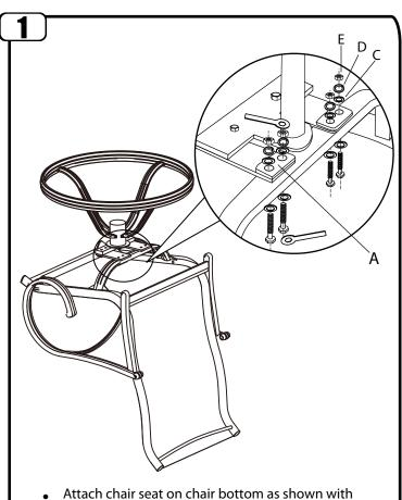
Attach chair seat on chair bottom as shown with Bolts(B), Washers(C), Backup Plates(A), Spring Washers(D) and Nuts(E).
