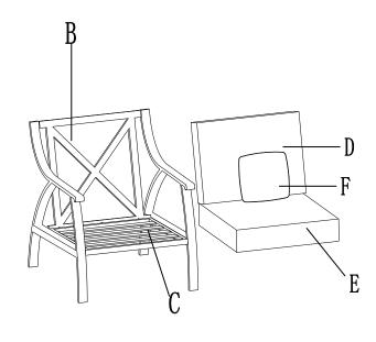
Step 3: Align the hole on Seat Board (C) with the hole on Rear Panel (B), then connect them by Bolt (BB), Spring Washer (DD) and Flat Washer (CC). Lock them tightly.
