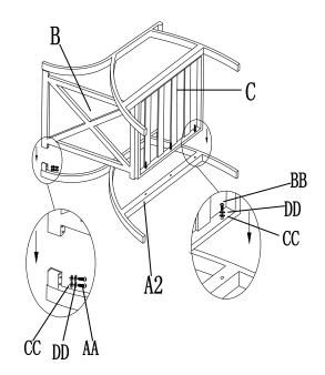
Step 2: Connect Seat Board (C) and Left Armrest (A2) by Bolt (BB), Spring Washer (DD) and Flat Washer (CC). Insert Rear Panel (B) into Left Armrest (A2) and lock them by Bolt (AA), Spring Washer (DD) and Flat Washer (CC). DO not lock tightly.
