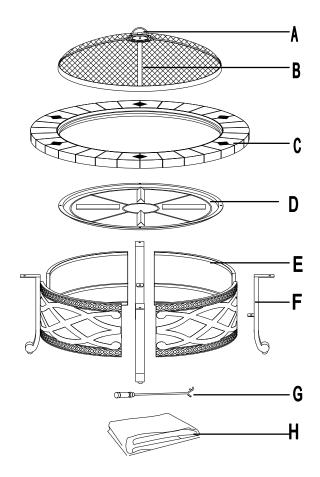
Step 1: Lock Screen Handle (A) with Lid (B) by Nut (AA) tightly.
