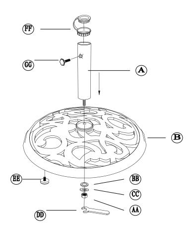
Step 1: Insert Umbrella Pole (A) into Umbrella Base (B). Firmly attach and tighten them together with Nut (AA) Flat Washer (BB) and Spring Washer (CC) by using Wrench (DD). See as picture. Assembly Completed!
