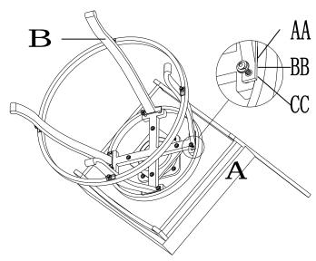
Step 2: Use Bolt (AA), Spring Washer (BB) and Flat Washer (CC) to connect Legs (B) and Chair Seat (A) by Wrench (EE) to lock all the parts tight.
