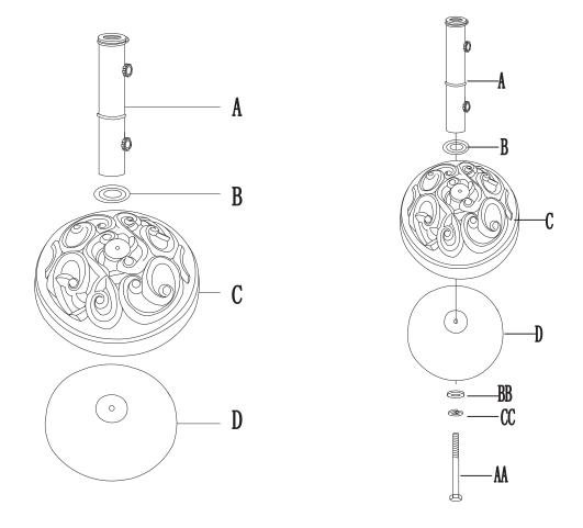
**Step:** Put Base (D) under the Umbrella Base (C), then put Plastic Washer (B) on the circle of the Umbrella Base (C), put Umbrella Pole (A) into Plastic Washer (B). Use Wrench (DD) to lock Bolt (AA), Flat Washer (BB), Spring Washer (CC) and Umbrella Pole (A) tight. Assembly Completed!
