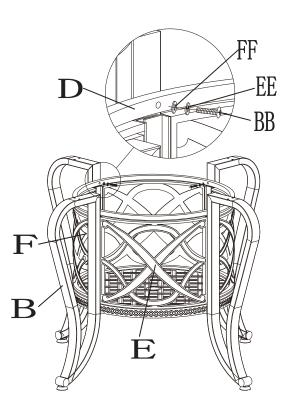
Step 2: Use Bolt (AA), Spring Washer (EE) and Flat Washer (FF) to lock Side Panel (E), Door Panel (F) and Leg (B). (Note: don't mess with the order. Put Door Panel in the middle, the Side Panel next to the Door Panel.) Assemble others in the same way. Don't lock tight.
