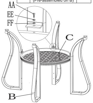
Step 1: Use Bolt (AA) ,Spring Washer (EE) and Flat Washer (FF) to connect Leg (B) with Bottom Fixed Ring (C). Don't lock tight.
