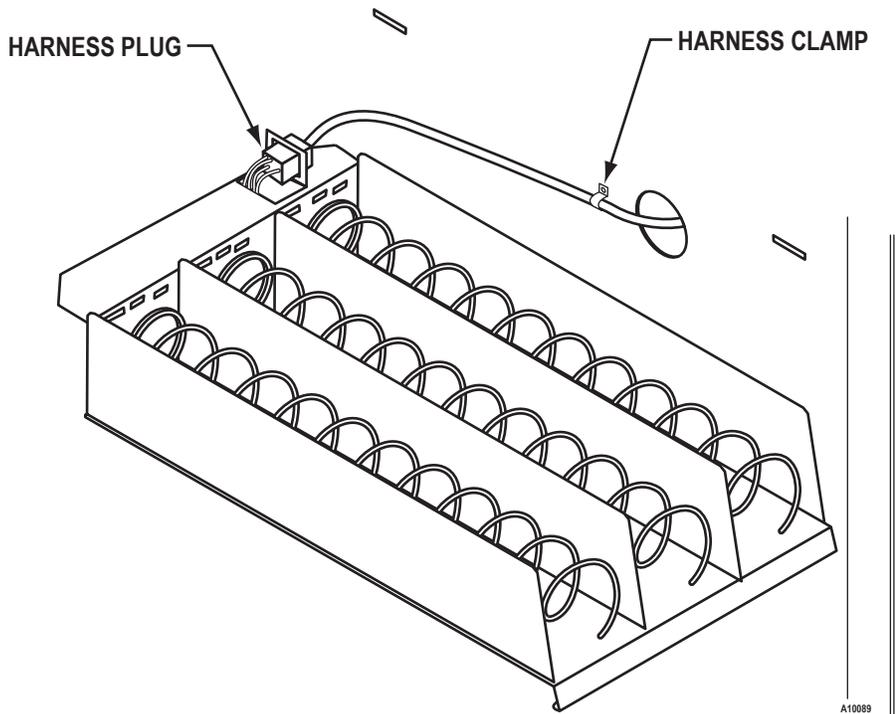
**FIGURE 4b. GF19 & GF35 TRAY HARNESS CONNECTIONS**
