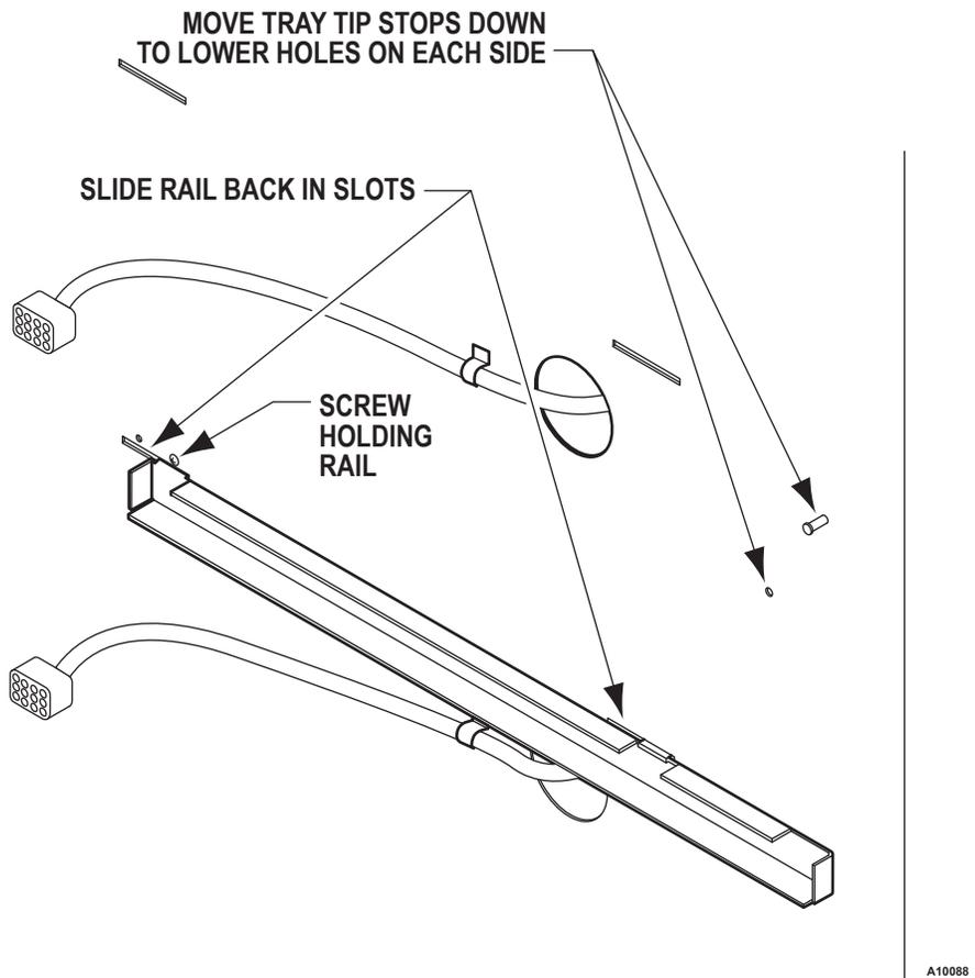
**FIGURE 4c. ADJUSTING A SIDE RAIL**
