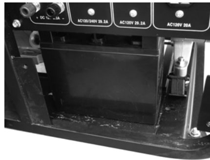
Connect battery and put in the cabin
