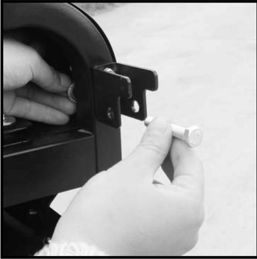
Install the handle bracket.
