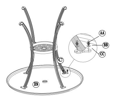
Step 2: Use Wrench (DD), Bolt (AA), Spring Washer (BB) and Flat Washer (CC) to connect Foot (C) and Table Top (B).
