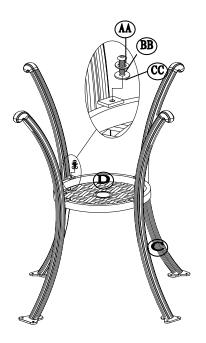
Step 1: Use Wrench (DD), Bolt (AA), Spring Washer (BB) and Flat Washer (CC) to connect Fixed Frame (D) and Foot (C). Don't lock tight.
