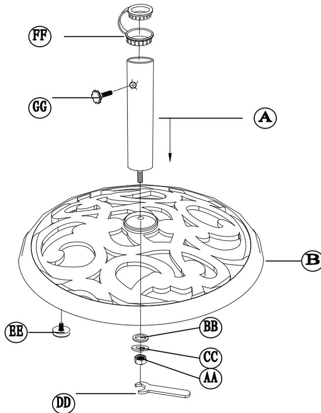
Step 1: Insert Umbrella Pole (A) into Umbrella Base (B). Firmly attach and tighten them together with Nut (AA) Flat Washer (BB) and Spring Washer (CC) by using Wrench (DD). See as picture. Assembly Completed!
