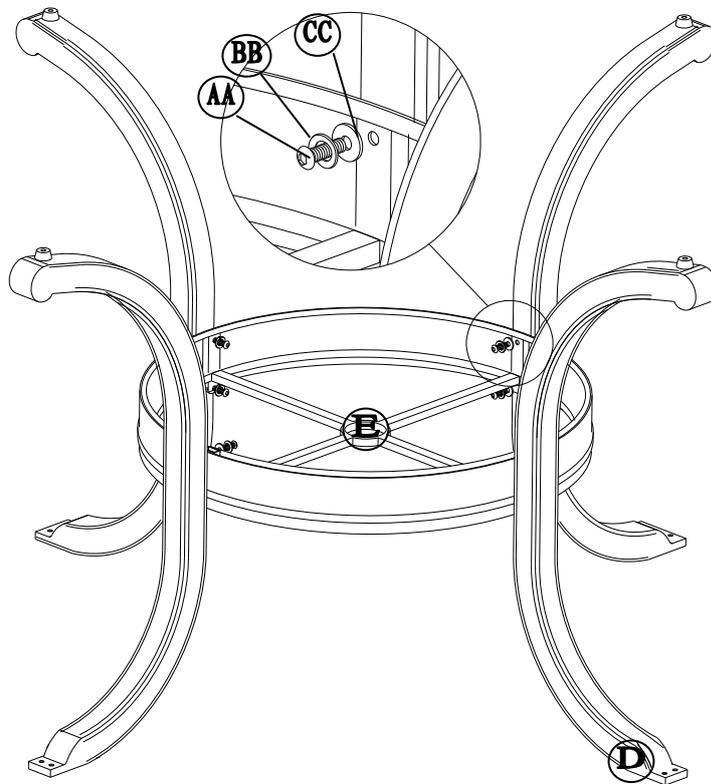
Step 1: Attach the Connecting Frame (E) to Leg (D) with Bolt (AA), Spring Washer (BB) and Flat Washer (CC) by using the Wrench (GG). Be careful do not lock tight.
