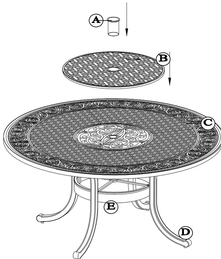
Step 3: Turn over the Table, tighten all the Bolts. (Adjust the Foot Pad slightly). Put Umbrella Hole Cap (A) and Swivel Plate (B) on Table Top (C). Swivel to adjust the Plate (B).
