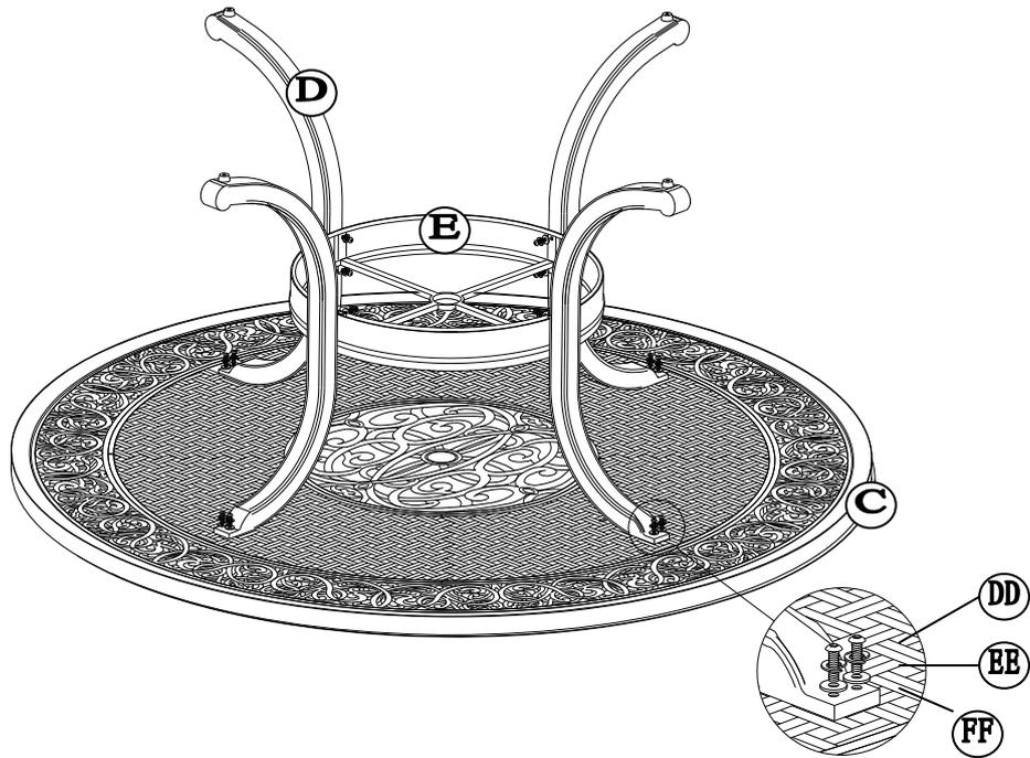
Step 2: Attach the Leg (D) to Table Top (C) with Bolt (DD), Spring Washer (EE) and Flat Washer (FF) by using Wrench (HH) to lock tight.
