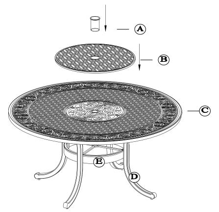
Step 3: Turn over the Table, tighten all the bolts. (Adjust the Foot Pad slightly). Put Umbrella Hole Cap (A) and Swivel Plate (B) on Table Top (C). Swivel to adjust the Plate (B). Assembly completed!
