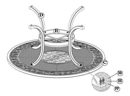
Step 2: Attached the Leg (D) and Table Top (C) using Bolt (DD), Spring Washer (EE) and Flat Washer (FF) by using Wrench (HH) to lock tight.
