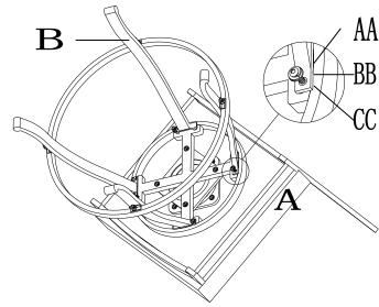
Step 2: Use Bolt (AA), Spring Washer (BB) and Flat Washer (CC) to connect Legs (B) and Chair Seat (A) by Wrench (DD) to lock all the parts tight.
