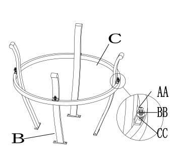
Step 1: Use Bolt (AA), Spring Washer (BB) and Flat Washer (CC) to connect Legs (B) and Under Fixed Ring (C). Do not lock tight.
